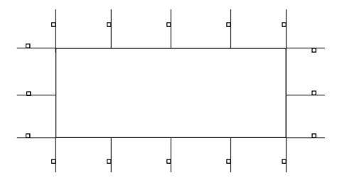
3rd: Assemble and lay out all tent poles which are made up of two pieces next to each rope. Also assemble the center poles made up of 4 sections each.
